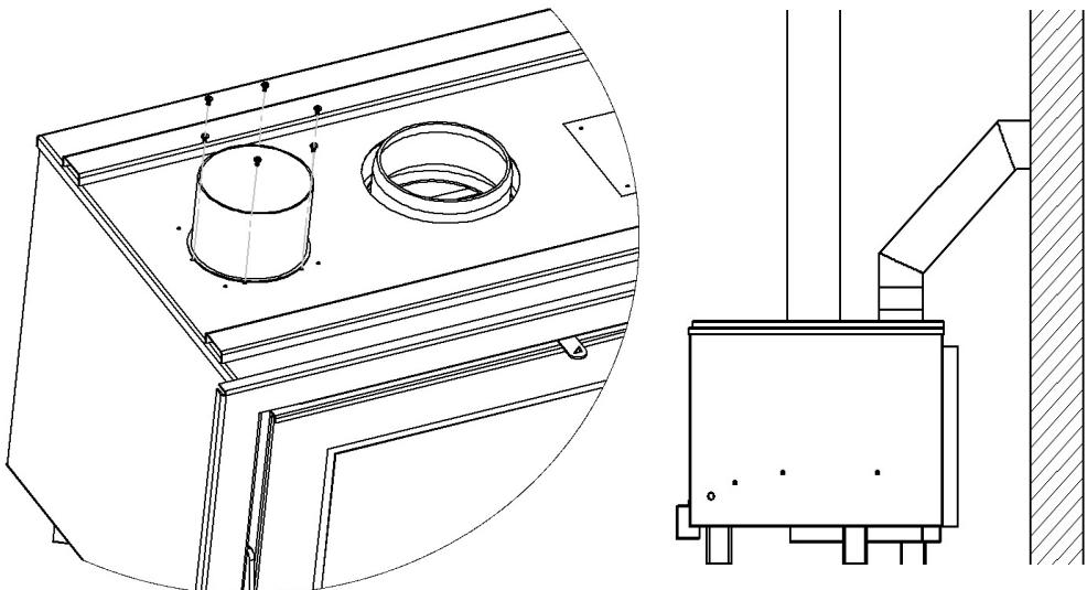
Every insert goes with 2 connectors, included inside, which are used to connect tubes to the appliance, by which hot air can be transferred to another room. The connectors are installed by removing the 2 lids on the upper surface of the insert (held into place by 4 screws) and fixing them in the same as the lids. (This time with 6 screws.)
